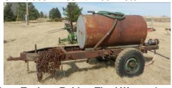
• 300 Gallon Water Tank on Rubber Tired Wagon (truck frame)
